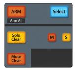
**Channel Controls.** Each channel is equipped with its own Select, Mute, and Solo buttons. When Arm is active, the Select buttons will turn red and will arm the tracks for recording. Solo and Mute Clear are also provided to quickly disable hidden solos and mutes.
