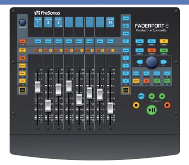
**Thank you** for purchasing the PreSonus® FaderPort™ 8 production controller. Featuring eight ultra-smooth, touch-sensitive, motorized faders; digital scribble strips; complete automation and transport controls; and the unique Session Navigator, the FaderPort 8 makes mixing in and controlling your favorite DAW application quick and easy.
