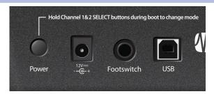
**Power and Power Switch.** This is the connection for your external power supply. Use the button to turn your FaderPort 8 on or off.
