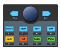
**Session Navigator.** These buttons alter the functions of the push-button encoder and the Next and Prev buttons on either side. Mackie Control users can press Shift with any of these buttons to access their function buttons:
