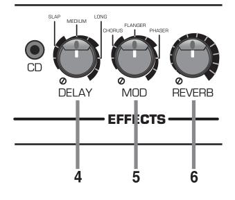
**6. REVERB:** Use this control to adjust the amount of digital reverb effect. In its fully counterclockwise position, the signal will be "dry" (without reverb). As you rotate this control clockwise, the amount of reverb increases.
