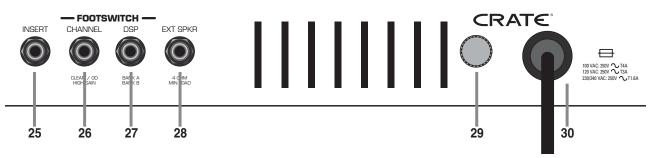
**25. INSERT:** Use this jack to connect an external signal processor to the amplifier. Use Crate's STP201, STP202, or STP203 stereoto-mono Y-cord or an adapter such as Crate's YPP117 and two 1/4" mono signal cables to connect to the effect, as shown below.
