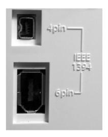
The FW-1804 is supplied with a 2 m (6-foot) cable. If you wish to use a longer cable, the length should not be more than 4 m (13 feet) and the cable should be the best possible quality available to avoid data loss, which results in audio dropouts.
