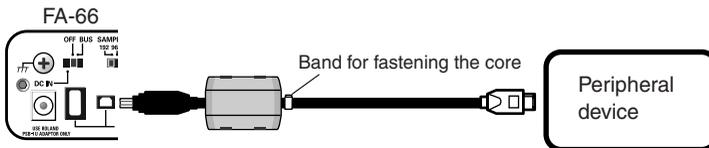
\* Be careful not to pinch your fingers when attaching the ferrite core.
