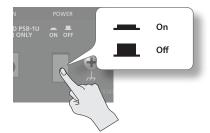
\* This unit is equipped with a protection circuit. A brief interval (a few seconds) after turning the unit on is required before it will operate normally.
