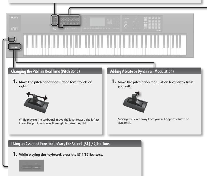
The sound changes according to the functions that are assigned to the [S1] [S2] buttons.
