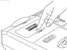
When you open the sample memory (RAM) slot cover, be careful not to press it too far backward. If you apply excessive pressure, the cover may come off and be damaged.
