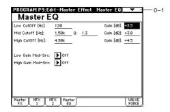
The MEQ High Gain and MEQ Low gain can be controlled by assigning a modulation source to the "Low Gain Mod-Src:" and the "High Gain Mod-Src:" functions on this page.
