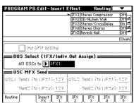
If you are connecting the Insert Effects in series, **check** the "**Chain**" box (Program P8: 8–2a). If you check the box that is located between IFX1 and IFX2, the output signal from IFX1 is sent to IFX2. When the Insert Effects are connected in series, the values of the "Pan (CC#8)," "BUS Select," "Send1," and "Send2" parameters for the post-IFX signal will be used (\*\*\*\* "3. Mixer").
