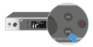
The receiver's display shows that the synchronization process has started.
