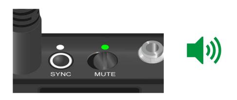
▷ Slide the mute switch to the desired position to mute or activate the audio signal.
