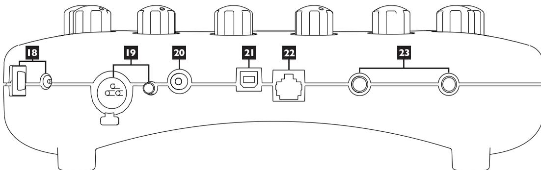
**18. Power** – connect the included PX-2 power pack and flip the switch here to bring your POD X3 to life.
