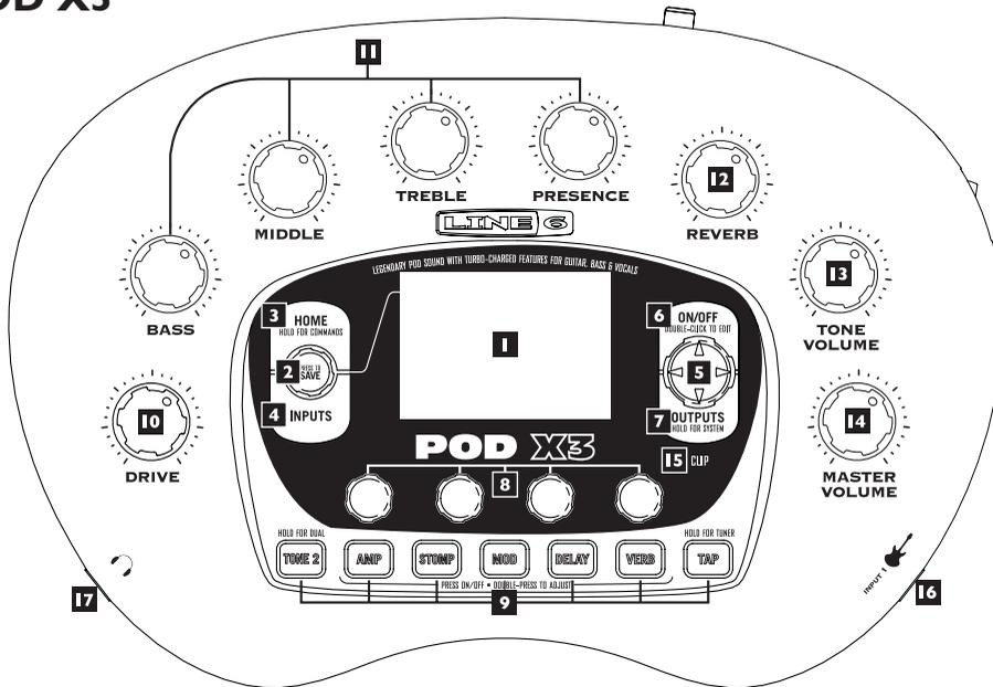
**I. Display** – the LCD (*liquid crystal display*) is your window into the power of POD X3. You’ll see (2) types of “pages” in the display:
