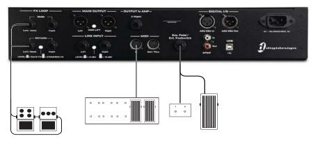
Figure 7. Effects and foot controller connections
