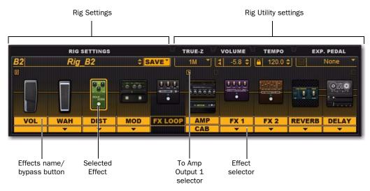
Figure 11. Eleven Rack Control window (in Pro Tools LE)
