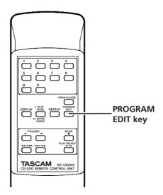
The unit enters program setting mode, and if no program has been set, it will be possible to set a track to program step 01 (MEMORY indicator blinks).
