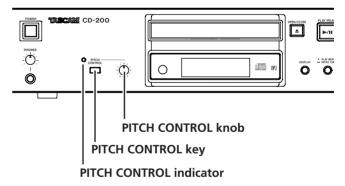
1 Press the PITCH CONTROL key on the main unit to turn pitch control playback ON.
