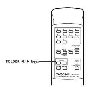
When using a data CD, by pressing the **FOLDER**  $\blacktriangleleft/\triangleright$ keys on the main unit or the remote control, you can skip to the previous or next folder. This will skip to the beginning of the first track in the previous or next folder. If you hold down one of these keys, you can skip through folders continually.
