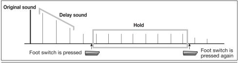
will activate hold, causing the current delay sound to be repeated (see illustration below). Pressing the foot switch once more cancels the hold condition, and the delay sound will decay normally.
