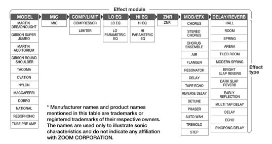
For some effect modules, you can select an effect type from several possible choices. For example, the MOD/EFX module comprises CHORUS, FLANGER, and other effect types from which you can choose one. The MODEL module is an effect for simulating the sound of various types of acoustic guitars. Switching effect types here means selecting different guitar body sounds.
