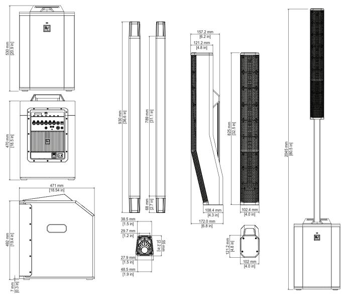
Figure 10.2: Dimensions EVOLVE50M System
