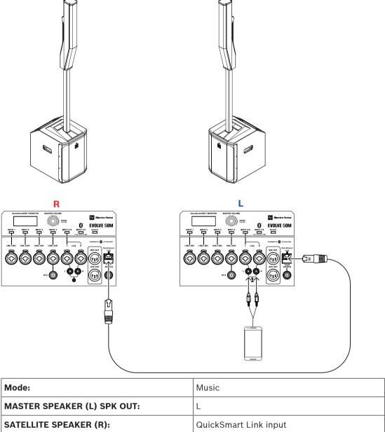
Tab. 8.4: DSP settings for the portable column system
