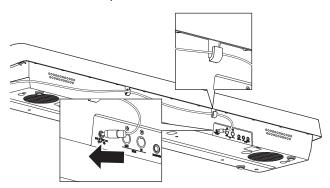
Connect the AC power adaptor to an AC outlet.
