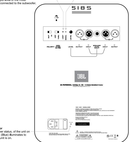
**POWER Indicator** Indicates AC power status, of the unit on and off. The LED (Blue) illuminates to indicate that the unit is on.
