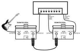
This diagram on the shows how to LINK two Decimator II pedals allowing the second pedal to track the direct instrument input. This will allow the second pedals' internal level detector to track the guitar directly, providing tracking performance similar to the professional rack mount Decimator ProRack G. Connect an RTS 1/8 inch cable from the LINK OUT of the first pedal to the LINK IN of the second pedal.
