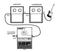
For best performance place all gain pedals in front of the Decimator II. You can put Delay and Reverb effects pedals after the Decimator II to avoid cutting off reverb and delay tails. NOTE: When connecting the Decimator into the effects loop of your amplifier connect the send to the Decimator II Input and return to Decimator II Output.
