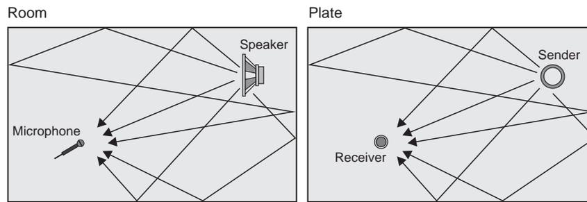
Fig. 4.2: Room reflections and reverb plate reflections
