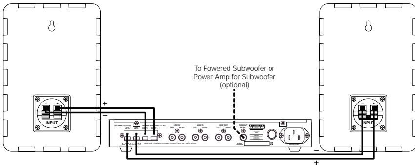
3. Connect the SUBWOOFER (optional). Connect the SUB OUT MONO jack to a powered subwoofer speaker system or to an amplifier powering a subwoofer speaker. Because this is a line level output, a shielded cable must be used for this connection. The SUB LEVEL regulates the volume to the subwoofer after the MASTER VOLUME Control. Adjust the SUB LEVEL control until a good blend between the subwoofer and speakers is achieved.
