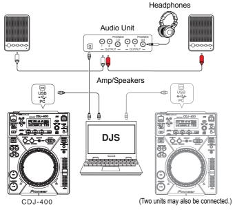
•Configuration when using an External DJ mixer (Example of Connections)
