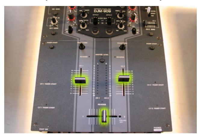
Gently pull the fader caps off the 2 channels and the crossfader.
