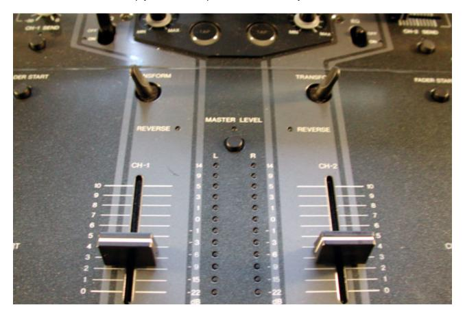
This picture shows my reversed / 90degree transform switches in the "cut" position.
