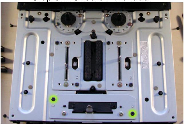
Remove the two black screws from opposite corners of the crossfader.
