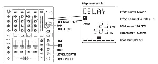
Beat effects allow the instant setting of effect times in synch with the BPM (beats per minute), thus allowing the production of a wide variety of effects in synch with the current rhythm, even during live performances.
