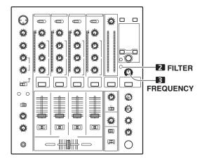
The effect frequency filter is linked to the **FREQUENCY** dial. The beat effect is applied only to the selected frequency band.
