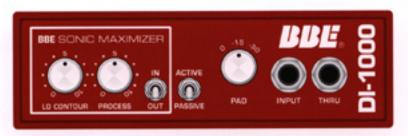
The PAD switch offers input attenuation of up to 30db allowing the "speaker output" of a guitar or bass head to be taken directly to a console input.
