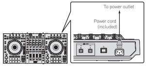
6 Press the  $[\Phi]$  switch on this unit's rear panel to turn this unit's power on.
