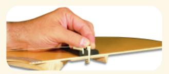
You might occasionally encounter an older guitar with a thin bridge or a string with a longer double winding adjacent to the ball end. Shown above is an old luthier's trick or remedy. An extra ball from an old string is placed over the string and drawn against the first ball. This will effectively back the string into the bridge, removing the heavy area of the string from direct saddle contact.
