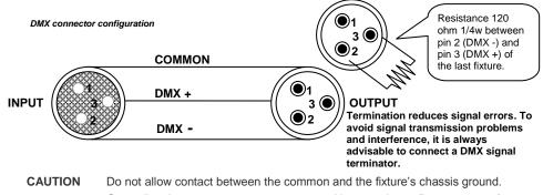
Grounding the common can cause a ground loop, and your fixture may perform erratically. Test cables with an ohm meter to verify correct polarity and to make sure the pins are not grounded or shorted to the shield or each other.
