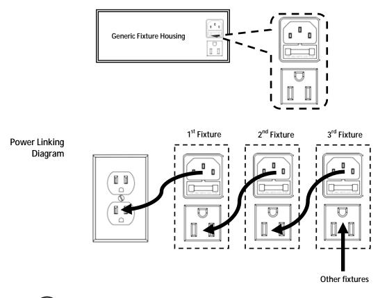
You can power link up to 11 Intimidator™ Spot LED 150 units on 120 VAC or up to 20 Intimidator™ Spot LED 150 units on 230 VAC.
