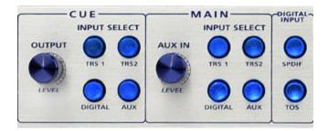
The CENTRAL STATION is loaded with separate CUE and MAIN signal paths. The CUE signal path includes the TALKBACK microphone signal and is intended for sending this signal to the recording artist via external headphone amp, or the two on board headphone amp. The MAIN signal path is intended for the "control room" and does not include the TALKBACK signal. (See application diagram for recording on page.)
