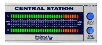
The CENTRAL STATION is loaded with dual independent tri colored 30 segment LED's for metering of the audio signal. The scale is represented in both dBfs and dBu for use with both analog outboard equipment as well as digital audio workstations, sound cards and other digital processors.
