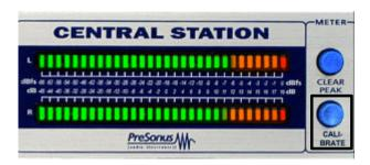
The meters of your CENTRAL STATION can be calibrated to match the meters in your DAW or other audio device. Note that the main audio path does not go through the meters of your CENTRAL STATION and the calibration procedure will not affect the sound of your unit.
