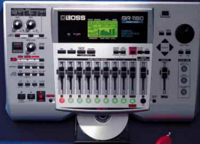
The BR-1180 Digital Recording Studio is more than a digital recorder, it's a complete music production system. You get 10 tracks of hard disk recording, 80 Virtual Tracks, onboard COSM® effects, a programmable Rhythm Guide drum track and an optional CD-R/RW drive for burning CDs (standard on the BR-1180CD). And because it's from BOSS, you won't lose your wallet—or your patience—owning one.
