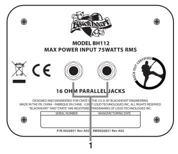
**1. 75W 16 Ohm Parallel 1/4" Jacks:** Connect the output of your amplifier (rated up to 75W into 16 ohms) to one of these jacks using good quality (non-shielded) speaker cable. Never use (shielded) instrument cable to connect speakers to an amplifier.
