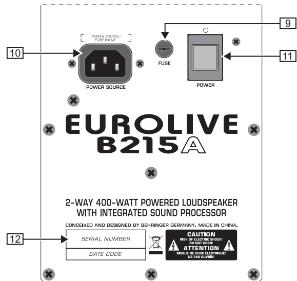
Fig. 2.2: Control elements and connections (B212A and B215A)
