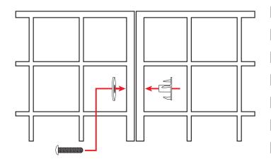
Repeat for each connection. Once all connections have been made, gently tighten each connection point using the supplied allen wrench. Do not over-tighten.
