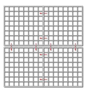
Staggered-Mounting: For staggered connections, mark **SpaceCoupler** (A) with the template. Drill holes. Position along side SpaceCoupler (B) according to desired pattern. Mark drill hole position for **SpaceCoupler** (B) through existing drill hole on **SpaceCoupler** (A).
