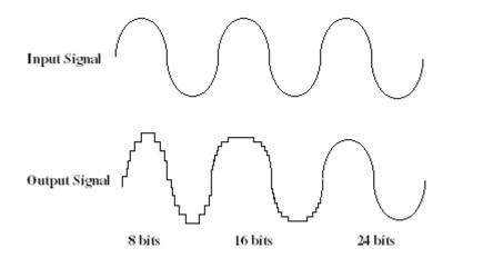
Figure B. The more bits there are available, the more accurate the representation of the signal and the greater the dynamic range.
