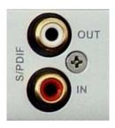
When connecting devices to the S/PDIF jacks, the use of standard analog RCA audio cables is not recommended. For reliable S/PDIF operation, 75-ohm coaxial (RG59) video cables are recommended.
