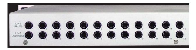
By default, the inputs and outputs are set to receive or send a +4dBu signal. You can switch between +4dBu and -10dBV for each individual input and output via the console software. (See section below).
