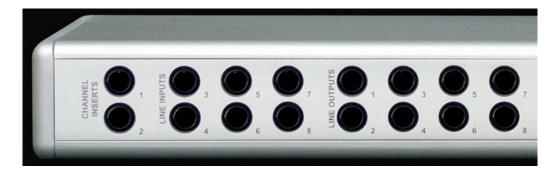
You can switch between +4dBu and -10dBV for each individual input and output via the console software (see section below). There are also two channel inserts on the rear panel where you can connect a serial effects device (compressor, EQ, etc.) for the universal inputs (1-2). The channel inserts are wired: tip = send, ring = return and sleeve = ground.
