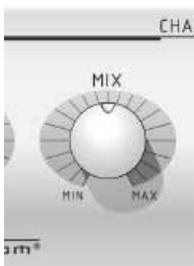
This control adjusts the amount of Big Bottom enhancement being added to the original signal. The lower the setting, the subtler the effect until there is no effect at all. The higher the setting, the more dramatic the effect.
