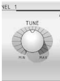
The Aural Exciter Tune control adjusts the corner frequency of the high pass filter, thus setting the range of frequencies being enhanced by the Aural Exciter. The range of the corner frequency is 800Hz (fully counter clockwise) and 6kHz (fully clockwise). The 12 o'clock setting is approximately 3kHz. As the tune control is adjusted clockwise, less and less mid-frequency enhancement will take place.
