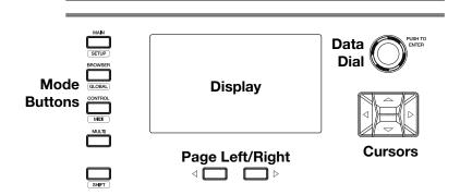
Advance 49's display shows information about its current mode and operations. You can navigate its different modes, pages, etc. by using the following controls:
