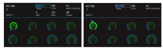
TypeThis determines whether the encoder sends a MIDI CC message or an<br/>increment/decrement message (Inc/Dec).CC#When Type is set to MIDI CC, this is the MIDI CC number that the encoder controls.<br/>The available range is 0–127.MIDI ChannelThis is the MIDI channel over which the encoder will send its MIDI message when you
