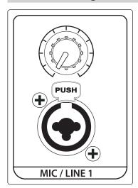
**Mic / Line input and level control**. Your AIR-series full-range loudspeaker is equipped with two Class A microphone preamplifiers for use with most dynamic microphone types. The combo connection on this input also supports a line-level signal.
