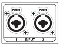
**Line inputs.** The AIR-series subwoofers feature two line-level inputs. These balanced XLR / ¼"TRS combo connections are provided to connect your subwoofer to a StudioLive-series mixer or other mixing console.
