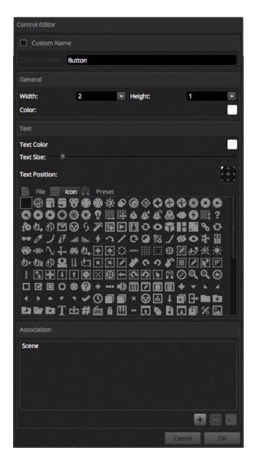
The association or pairing of a control can be edited by clicking 'Edit Association'. The Association window appears with a list of commands. Several commands may be added so that one button can be used to trigger several different scenes, or 1 fader can be used to control the speed of several scenes.
