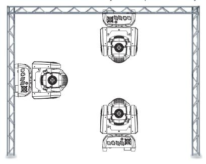
The Focus Spot Two is fully operational in three different positions, hanging upside-down from a ceiling or trussing, mounted sideways on trussing, or set on a flat level surface. Be sure this fixture is kept at least 0.5m away from any flammable materials (decoration etc.). Always use and install the supplied safety cable as a safety measure to prevent accidental damage and/or injury in the event the clamp fails (see next page).
