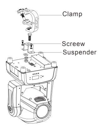
Screw one clamp via a M12 screw and nut to the included bracket. Attach the bracket using the omega locks to the bottom of the Focus Spot Two. Attach and pull the safety-cable through one of the safety holes located on the bottom base and over the trussing system or a safe fixation spot. Insert the end in the carabine and tighten the safety screw.
