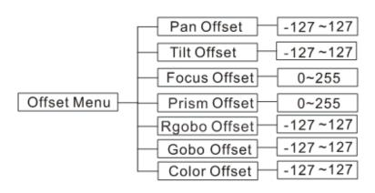
To enter the Offset Menu, press the MENU button to unlock the display, then press the ENTER button for at least 5 seconds. In this submenu you are able to adjust the home position of the pan, tilt, focus, prism, rotating gobo motor, gobo wheel, and color wheel. To exit this menu press and hold the MENU button.
