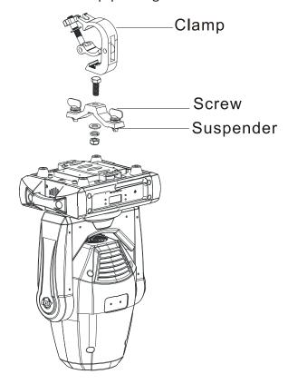
Screw one clamp via a M12 screw and nut to the included bracket. Attach the bracket using the omega locks to the bottom of the Focus Spot Three Z. Attach and pull the safety-cable through one of the safety holes located on the bottom base and over the trussing system or a safe fixation spot. Insert the end in the carabine and tighten the safety screw.
