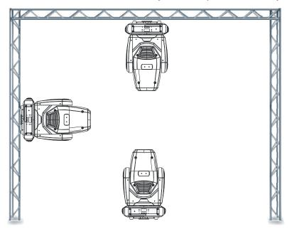
The Focus Spot Three Z is fully operational in three different mounting positions, hanging upside-down from a ceiling, mounted sideways on trussing, or set on a flat level surface. Be sure this fixture is kept at least 0.5m away from any flammable materials (decoration etc.). Always use and install the supplied safety cable as a safety measure to prevent accidental damage and/or injury in the event the clamp fails (see next page).
