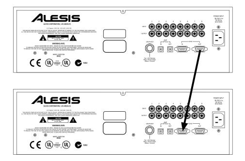
Power on the machines from first to last. If a BRC remote control is present, power it up after the ADATs.
