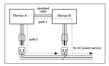
One path goes from device A to ground via the ground terminal of the three-conductor AC power cord, but A also sees a path to ground through the shielded cable and AC ground of device B. Because ground wires have a small amount of resistance, small amounts of current can flow through ground and generate a voltage along the cable shield. This signal may end up getting induced into the hot conductor.
