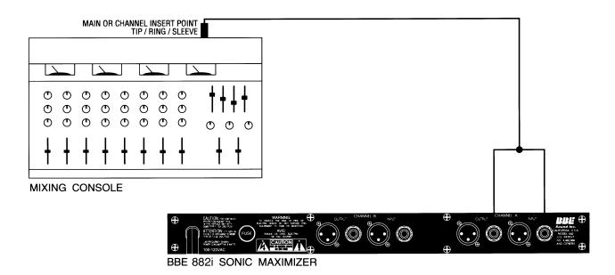
There are a couple of ways to configure the BBE 882i into a powered mixer. The ideal method would be into "Pre-Amp Out/Power Amp In" section of the console. If your console does not have this option, use the main or channel insert points.
