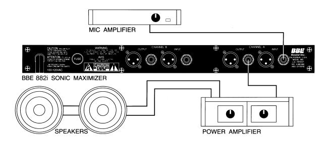
The BBE 882i will accept the output level of most sound contractor type mixers.
