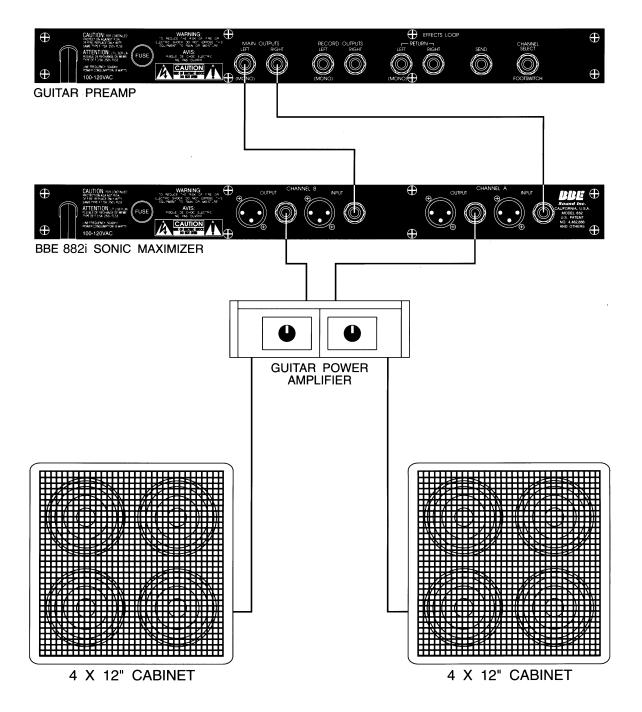
Use the BBE 882i in the effects loop or the main output of a guitar preamp. For keyboards, the output of the sub-mixer will be the ideal location.
