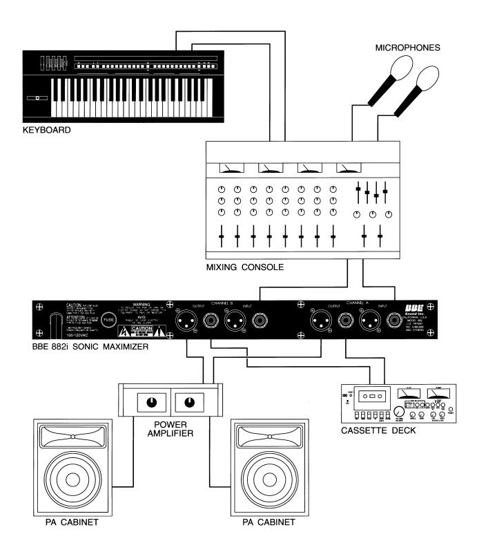
Connect the BBE 882i to the output of the mixing console. The output of the BBE will drive either a crossover or a power amplifier directly. (If an equalizer is being used, refer to "BBE and Equalization" section under "General Operation.")
