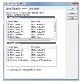
Figure 8-2: Activating the MOTU audio WDM driver in SONAR by highlighting 828mk3 inputs and outputs.
