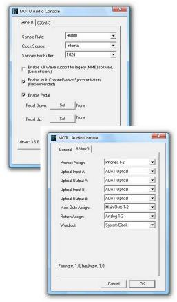
Figure 8-1: MOTU Audio Setup gives you access to all of the settings in the 828mk3 hardware, including the clock source, sample rate and optical I/O enable/disable.
