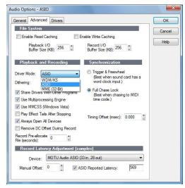
Figure 8-3: Enabling the ASIO driver instead of the WDM driver.
