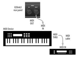
Figure 4-10: Connecting additional devices with MIDITHRU ports.
