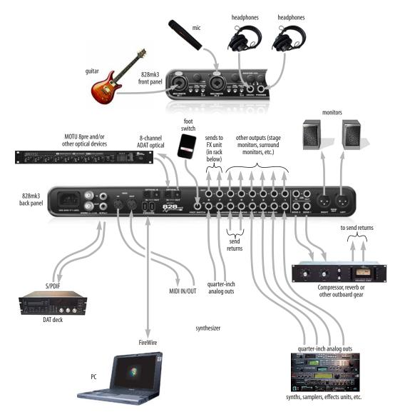
Figure 4-11: A typical 828mk3 studio setup.
