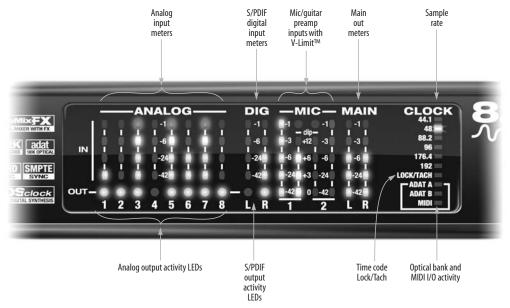
Figure 6-2: The 828mk3 front panel meters and LEDs.
