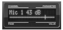
Figure 4-4: The LCD gives you feedback as you turn the TRIM knobs for the two mic/quitar inputs.
