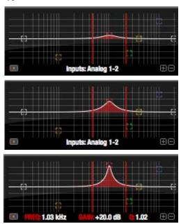
Figure 11-14: Type II EQ filter style.
