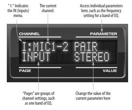
Figure 6-6: The IN (inputs) menu.
