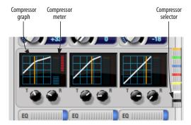
Figure 11-5: The Compressor controls.
