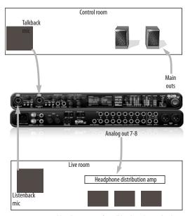
Figure 11-25: Typical hardware setup for Talkback and Listenback.
