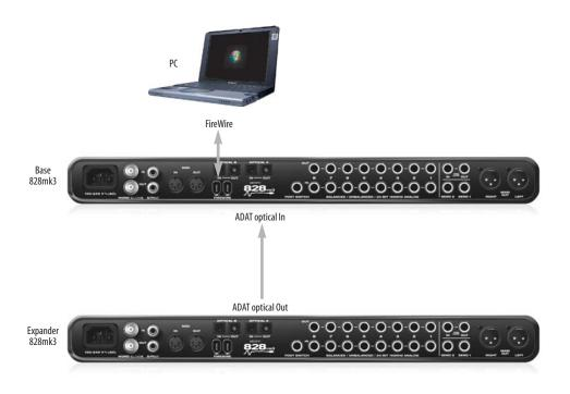
Figure 4-12: Using the 828mk3 as an optical expander. In this example, it is connected to another 828mk3.
