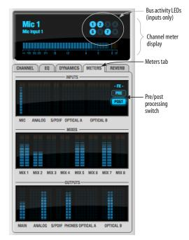
Figure 11-22: The Meters tab.
