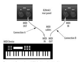
Figure 4-9: Connecting a MIDI device to the 828mk3.
