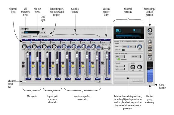
Figure 11-1: CueMix FX is a virtual mixer that gives you control over the 828mk3's on-board mixing features.
