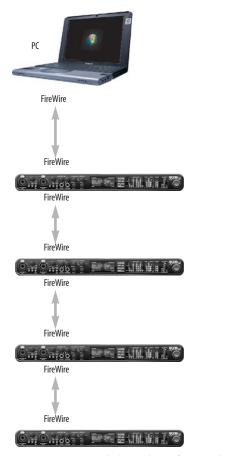
Figure 4-21: Connecting multiple 828mk3 interfaces (or other MOTU FireWire audio interfaces) to a computer.
