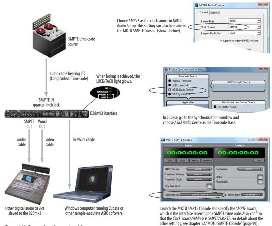
Figure 4-16: Connections for synchronizing the 828mk3 directly to SMPTE time code.
