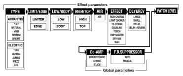
The parameters TYPE, LIMIT/EDGE, LOW/BODY, HIGH/TOP have separate settings for acoustic and for electric guitar. Depending on whether ACOUSTIC or ELECTRIC is selected for the TYPE parameter, the content of the other three parameters changes as follows.
