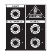
Fig. 2.9: Monitor/main mix connectors
