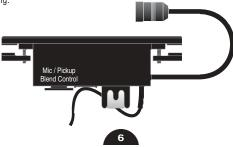
Balance between the microphone and magnetic signals is controlled by a small rotary blend control, located underneath the pickup. Move the wheel towards the treble strings for more pickup, and towards the bass strings for more microphone.
