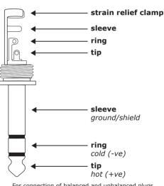
For connection of balanced and unbalanced plugs, ring and sleeve have to be bridged at the stereo plug
