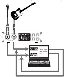
When Loopback is enabled and "Virtual" is selected in Universal Control, the audio from another application will be recorded on the last pair of driver inputs (Studio 26c: 5/6, Studio 68c: 7/8).
