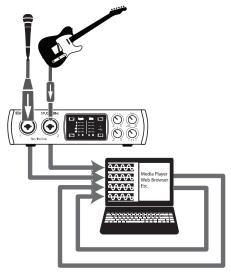
**Power User Tip:** When using either option, it's important to avoid creating a feedback loop. To do this, you'll need to have your monitors or headphones connected to Outputs 3/4 of your interface instead of Outputs 1/2,
