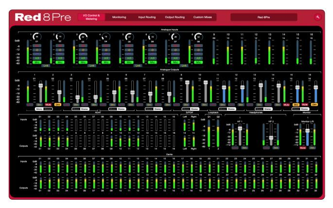
**Analogue Input** – Channel controls operate in the same manner as RedNet devices – See page 9 for details. For channels with gain controls and input functions, the level meter indicates the post-processing signal.
