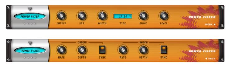
The **Power Filter** was developed in cooperation with GMedia and is based on their famous impOSCar filter design. This rich-sounding filter requires a fair amount of CPU power and should be used sparingly on slower computer systems. It's the same Power Filter as the one in the Filter section, but with more filter types and an additional dedicated LFO for sweeping the width, which is useful for producing formant and vowel sweeps.
