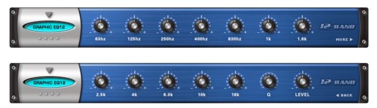
The **Graphic 12-Band EQ** is useful for tailoring a full spectrum audio source with fine controls of multiple bands for precision control. With the Q control, it's more versatile than an average graphic EQ — it is capable of comb filter FX and even basic speaker simulation effects.
