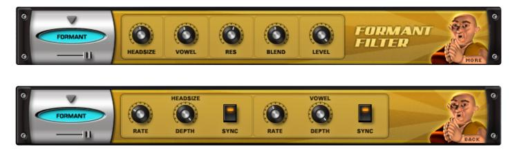
The **Format Filter** adds characteristics of the human voice to any sound. It accomplishes this by chaining a narrow set of bandpass filters, set at specific frequencies, which reflect the formants of the human voice.
