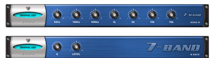
The **7 Band Graphic Equalizer** is useful for tailoring a full spectrum audio source with broad control of multiple bands. With the Q control, it is much more versatile than an average graphic EQ — capable of achieving comb filter FX and even basic speaker simulation effects.
