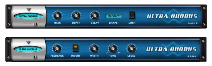
Chorus is a pitch and delay effect that adds a rich, shimmering quality to a sound by detuning and delaying the incoming signal and combining it with the unaffected signal. The **Ultra Chorus** has a dedicated LFO—a 'LUSH' control, which gives this unit a dense, rich character.
