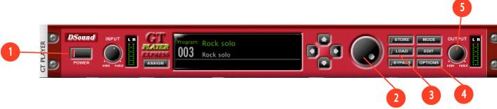
Click the Power button (1) on the effect rack and the button will light up. Use the Dial (2) to select the preset Rock Solo and click on the Load button (3). You can now play your guitar and hear the effects. The effects pedals used to create that preset will appear on the screen. Use your mouse to adjust the pedal parameter values. Use the Output knob (5) to adjust the volume.
