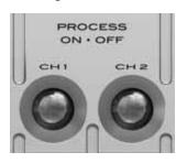
The IN position turns all processing on and sends Aural Exciter and Big Bottom enhancement to the outputs. The buttons glow green when processing is on. They are dark when processing is off. When processing is off, only the unmodified signal passes through to the outputs. Switching the button back and forth offers a quick A/B comparison, allowing you to hear the enhancements from the Exciter in your program content.
