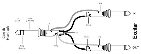
Note: Some manufacturers reverse the Tip and Sleeve connections, where the Tip is Return and the Sleeve is Send. This would mean that IN becomes OUT and OUT becomes IN when referring to the previous drawing. Be sure to check the owner's manual of your console.
